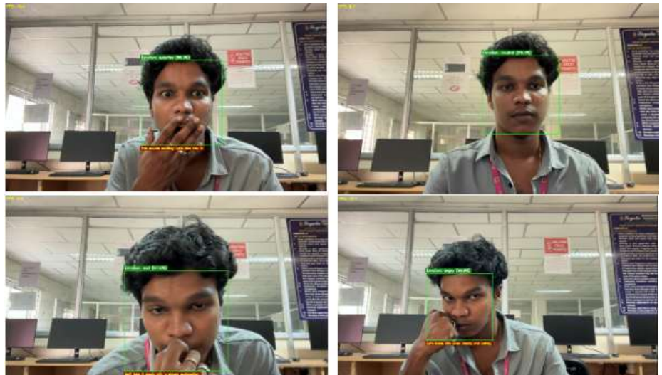
Figure 6. Real-time interface of the proposed emotion-aware AI system detecting and classifying learners' facial emotions during programming tasks for adaptive prompt generation.
